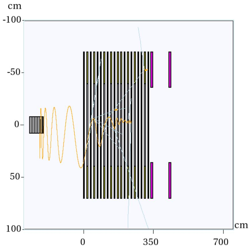
FIG. 15. 60 MeV electron traveling through tracker in XY direction; the photon emitted happens in the calorimeter (first run).
