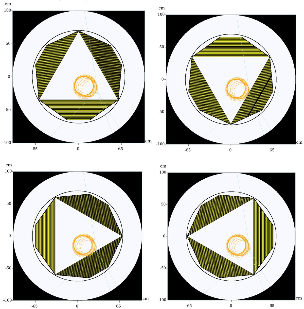
FIG. 16. 105 MeV electron sent through trapezoid panel tracker in toy model.
