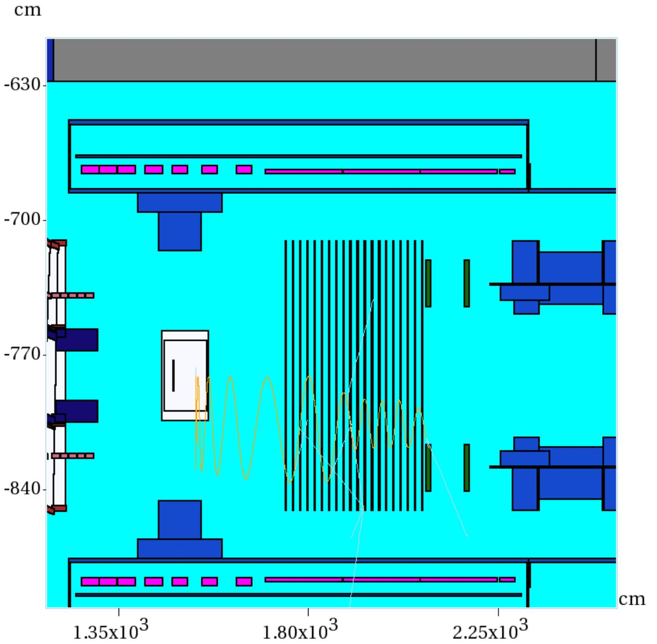
FIG. 19. 105 MeV electron moving through tracker and reaching first calorimeter.
