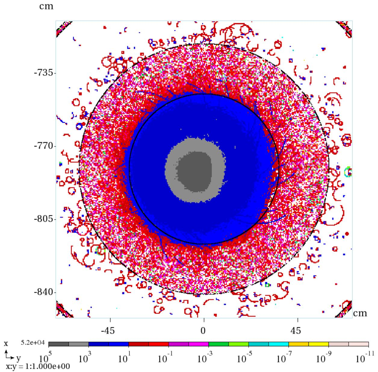
FIG. 25. Calorimeter disk 2 power deposition histogram.
