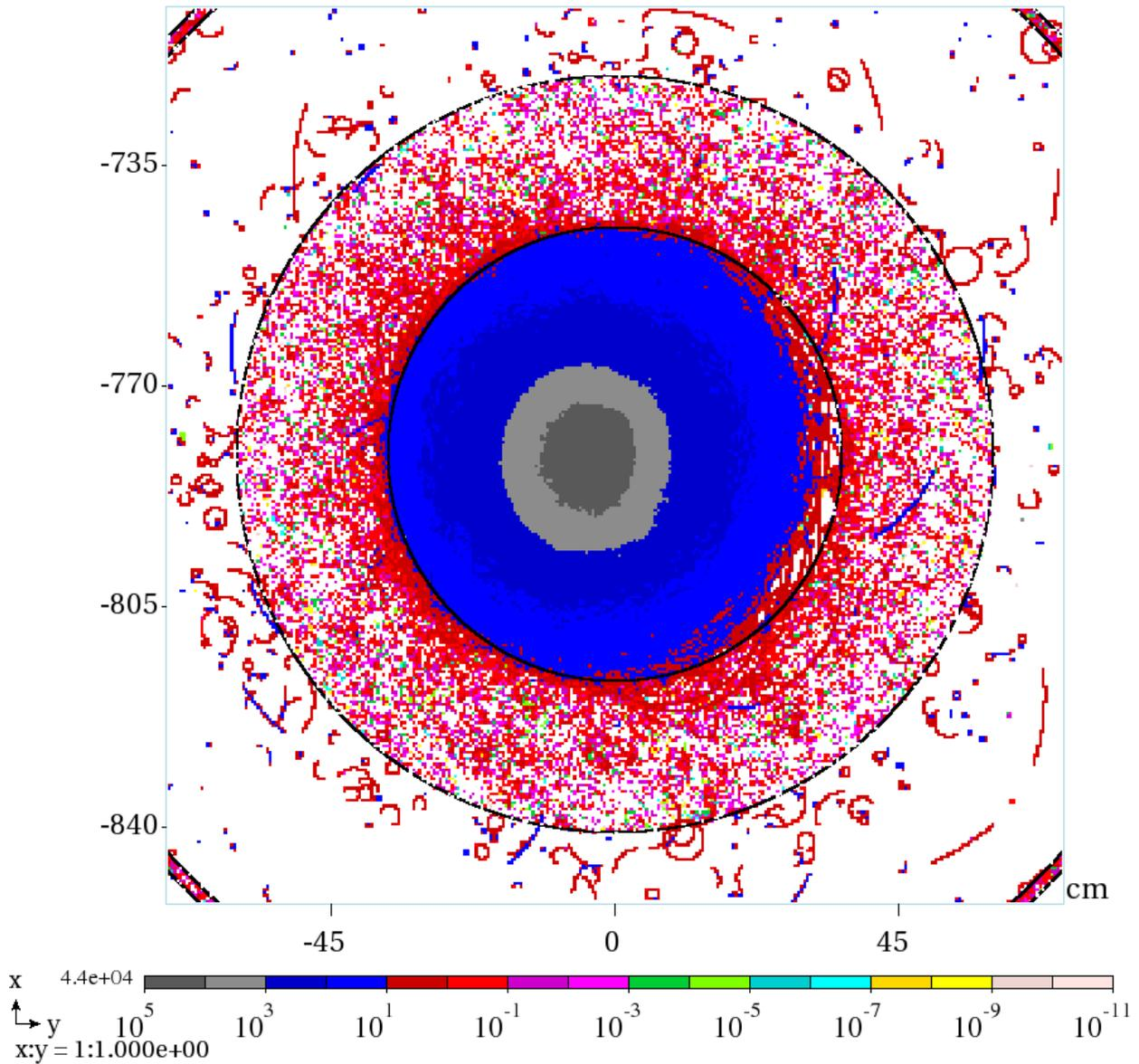
These histograms state that for the first disk, there is an average power deposition, also known as dose rate of 2.55 kRad/yr, while the second disk yields an average dose rate of 1.31 kRad/yr. The peak dose rate for the first disk is found to be approximately 22 kRad/yr, while the second disk has a peak dose rate of approximately 18 kRad/yr. The peak dose rates are found
